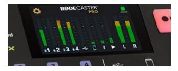
This indicates the input levels, i.e. whether the sound is saturated. They should generally be between -12 and -6. If the screen is in color, they are green or orange. If they are red, you need to turn the sound down.
